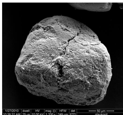
FIGURE 2 - Glauconite aggregate of round shape, SEM, 200X magnification
