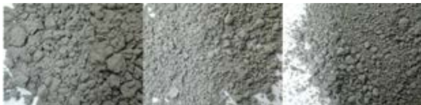
Fig. 1. Macroscopic analysis of fly ash FA2006, sodalite S and sodalite modified by chitosan S-CS
